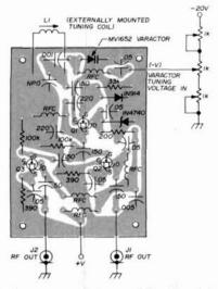
fig. 3. Component placement for the printedcircuit board used for the varactor tuned vfo. Full-sized PC board is shown in fig. 4.
